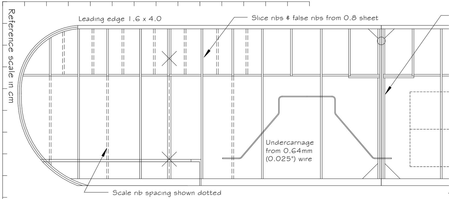
Wing spar 0.8 x 7.2. Lower rib sections are slotted into spar, upper rib sections are glued to top of spar.
